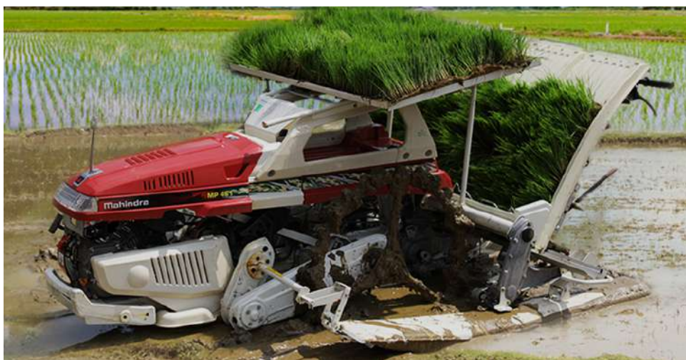
Fig. 69 Mechanical rice transplanter
