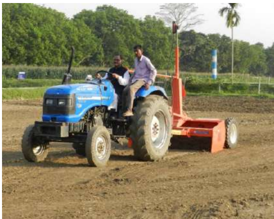
Fig. 68 Use of Laser Land Leveling
